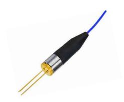
The FPLD series fiber-coupled laser diodes are designed with a GaAs quantum well structure. These diodes feature a built-in photodiode for precise monitoring and feedback control of the laser's output power. Housed in standard TO packages, these diodes are pigtailed to a 1-meter long single-mode fiber terminated with an FC/APC connector. Each unit undergoes rigorous testing prior to shipment to ensure reliability.
